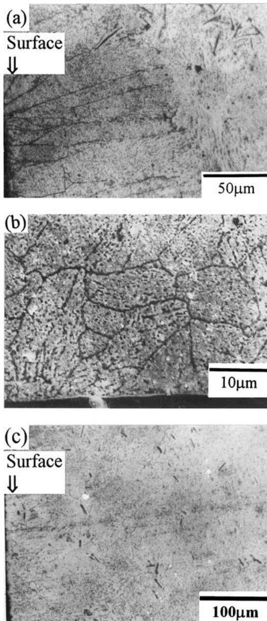
Figure 8 Morphology of Sn-9Zn-0.5Al aged 30 days (a) OM, (b) SEM, and of Sn-9Zn aged 30 days (c) OM.
