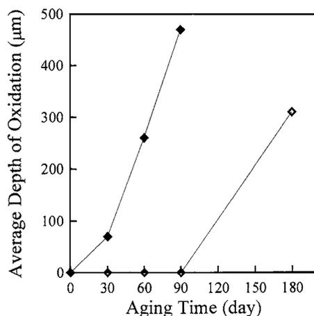
Figure 9 The depth of grain boundary oxidation of Sn-9Zn and Sn-9Zn-0.5Al.
