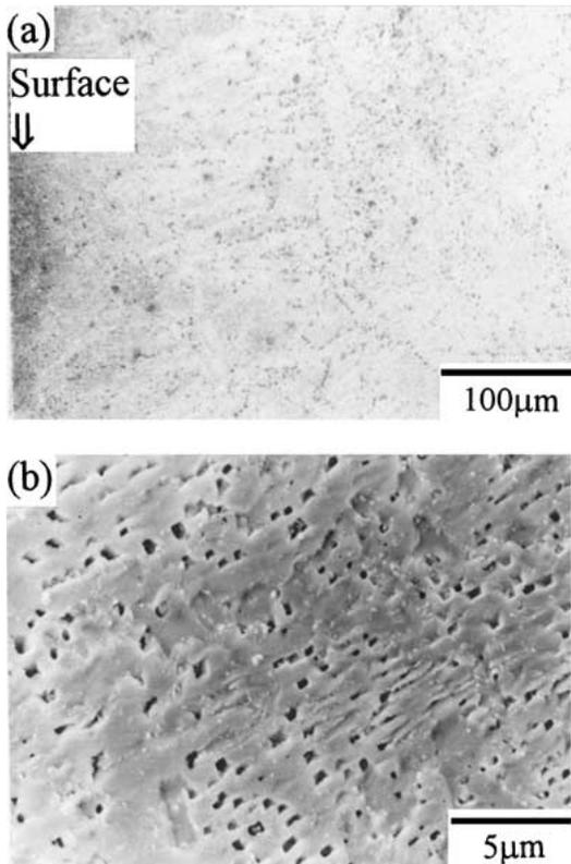
Figure 2 Microstructure of as-cast Sn-9Zn specimen: (a) OM, and (b) SEM.
