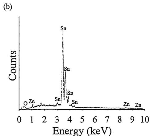
Figure 7 Typical EDS spectrum of Sn-9Zn after aged for 180 days: (a) in eutectic cell boundary, and (b) inside of eutectic grain.
