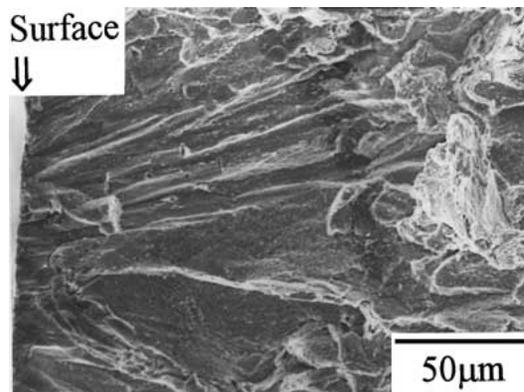
Figure 5 Fracture surface of Sn-9Zn-0.5Al aged for 30 days.
