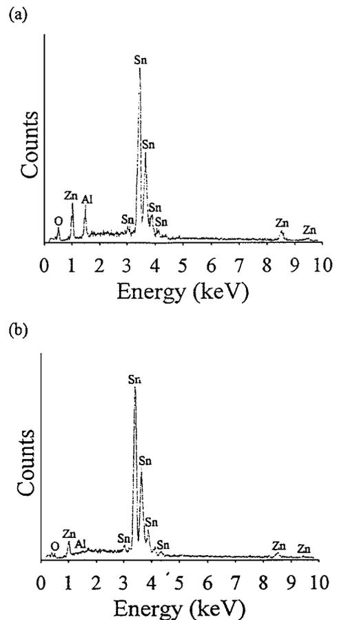
Figure 10 Typical EDS spectrum of Sn-9Zn-0.5Al after aged 90 days: (a) in eutectic cell boundary, and (b) inside of eutectic grain.
