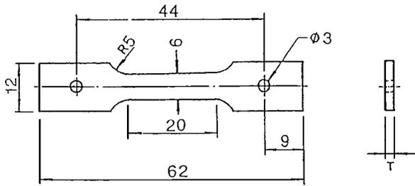
Figure 1 The dimension of tensile specimen (unit: mm).
