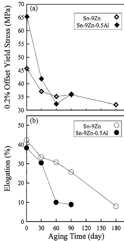
Figure 3 Tensile properties vs. aging time of Sn-9Zn and Sn-9Zn-0.5Al alloys: (a) 0.2% offset yield stress, (b) elongation.
