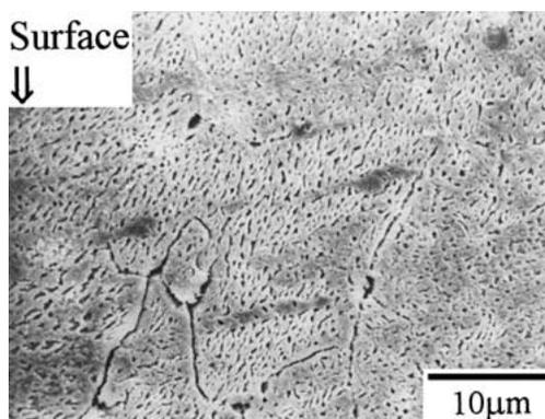
Figure 6 Morphology of Sn-9Zn after aged for 180 days.
