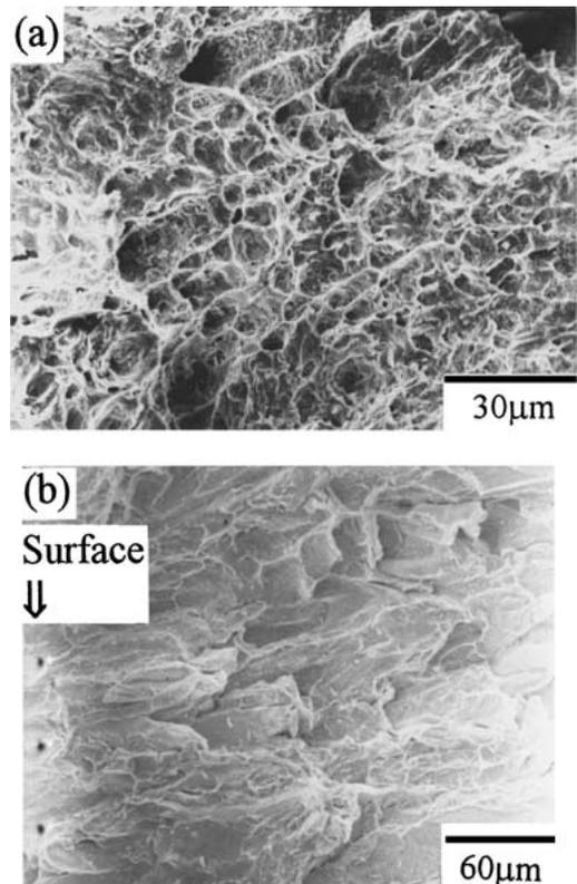
Figure 4 Fracture surface of Sn-9Zn: (a) as-cast, and (b) aged for 180 days.
